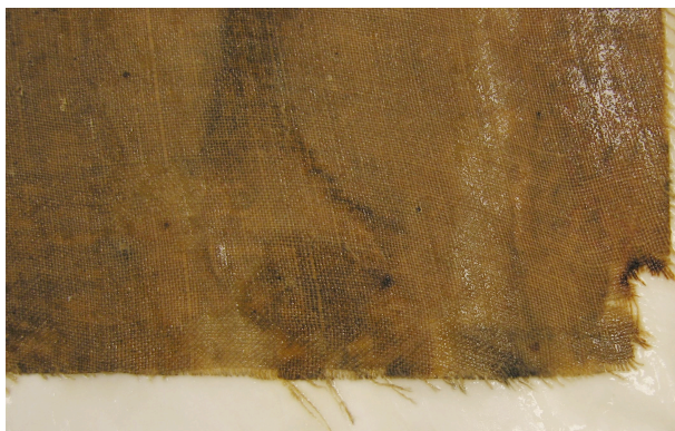
Fig. 2. Verso, detail of the frayed edges of a large, varnished map impregnated with SMC. Phelps & Ensign's travellers' guide, and map of the United States , 1837, 1840. Intaglio on wove paper, hand-colored. 0.745 x 1.05 m, Map Library, University of Michigan Library, no catalogue number.
