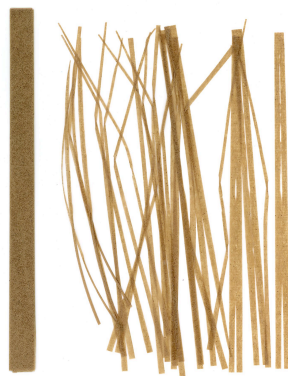
Fig. 1. Trial samples of remoistenable mending tissue for papyrus.
